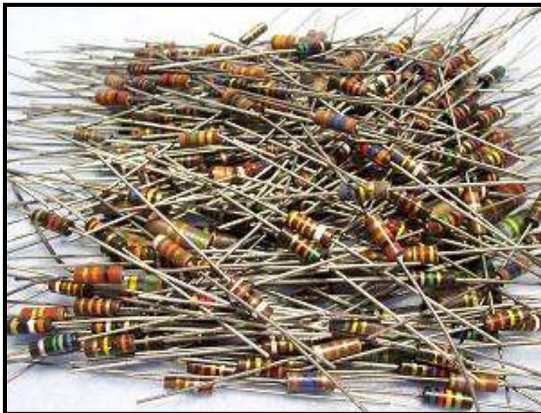
Resistors are non-polarized which means you can put them in either way.
