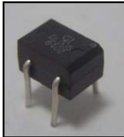
The leads are marked with “~” for the AC input and “+” and “-” for the positive and negative outputs. This is a very critical part that must NOT be installed incorrectly.
