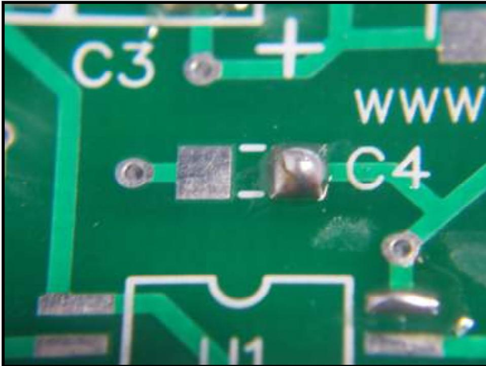
2. Solder one end of the component first.
